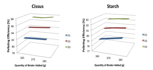
**Fig. 2a.** Surface Response of Pelleting Efficiency to Cissus Quantity and Pellets Diameter
