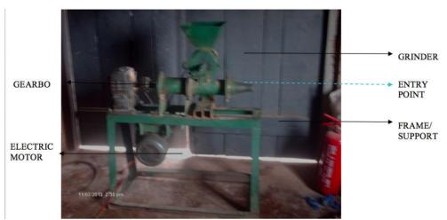
Plate 2: The Combined Grinding and Pelletizing Machine
